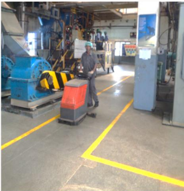
Fig.2.14 Special stone flooring to avoid slippery and easy cleaning with machines to improve hygiene
