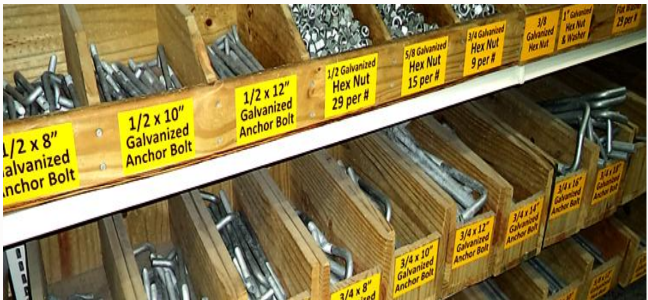
Fig 3.5 Allocated nuts, screws and bolts boxes in the facility to manually count them before and after the process in order to prevent their entry in food.
