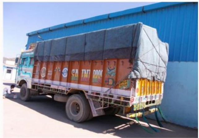
Fig 7.2. Multilayer Tarpaulin to protect from water and dust.
